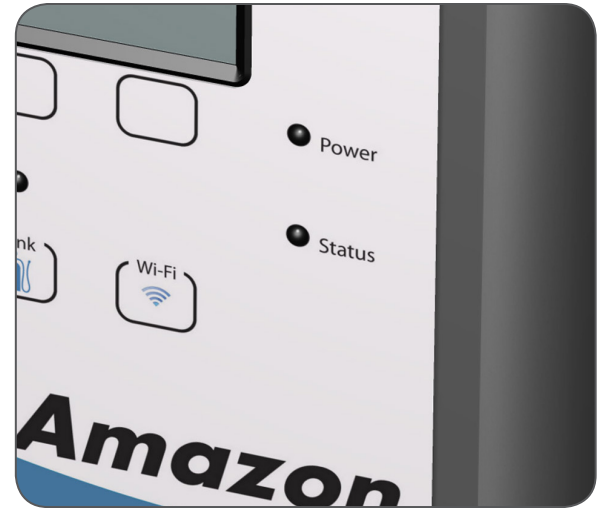
Wi-Fi button on front of the Amazon Bubbler
